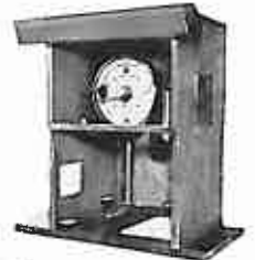
A filament must remain absolutely rigid when incandescent. To test this, current is switched on and the middle support removed.
