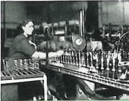
Inspecting the filament by projection on to a screen. The stem with the complete filament is examined before it is sealed to the bulb.
