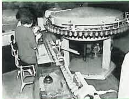
The capping machine. The operators are threading the leads through the cap.
