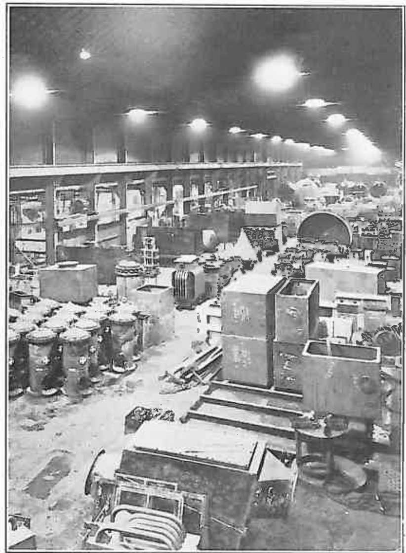
Large Engineering Erecting Shop lighted by 500 watt Mazda Lamps in Mazdalux Dispersive Reflectors.
