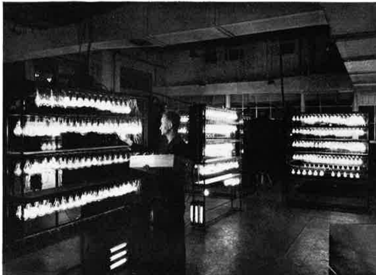
Left: Corner of Life Testing Room. Batches of lamps taken at random from each day's production are tested for life in this room. By running the lamps on excess voltage they can, in a few hours, be subjected to the same strain as in a normal life of 1,000 hours or more.
