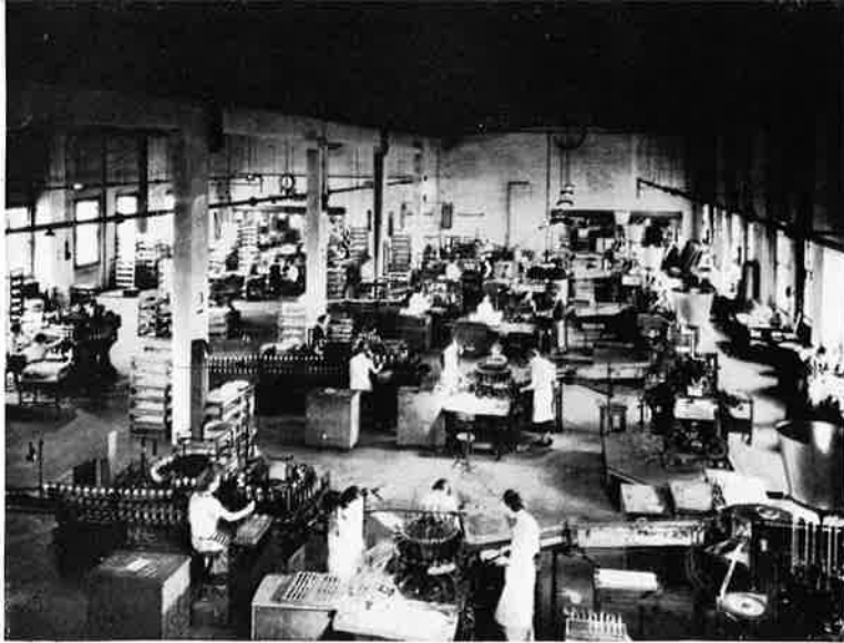
The Lamp Assembly Units in this section of the Mazda Lamp Works at Rugby comprise some of the most amazing automatic equipment so far employed in the manufacture of electric lamps. Machines of miraculous ingenuity and unerring accuracy carry out, at a high rate of speed, and with complete infallibility, intricate operations which can hardly be seen by the unaided eye.
