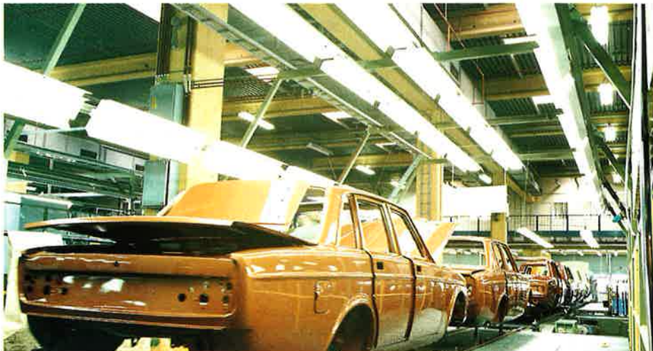
Cool White (Daylight UK) fluorescent lamps blend well with Natural Daylight, giving a cool appearance suitable for industrial applications.
