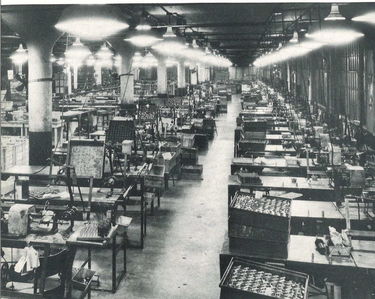
Workers in this modern radio factory enjoy 80 footcandles of light on their work. This splendid illumination is supplied by alternate units of High Intensity Mercury Lamps and 500-watt MAZDA lamps in Glassteel Diffusers spaced on 8' x 8' centers and mounted 9 feet above the floor.
